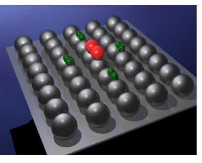
HTI's NxCat Catalyst is engineered to exhibit the "1-1-0" crystal orientation of its active catalyst metals, enabling the direct synthesis of hydrogen peroxide from hydrogen and oxygen, with little or no formation of water as a byproduct.
