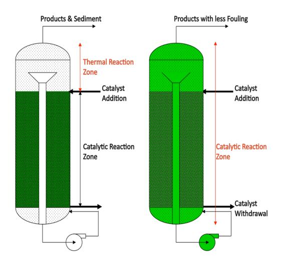
The ebullated bed reactor has been in commercial use for 40+ years. When HCAT is added, the full EB reactor volume is utilized for the conversion reaction. The solid catalyst can be optimized for enhanced functions such as HDS (desulfurization) and metals removal.
